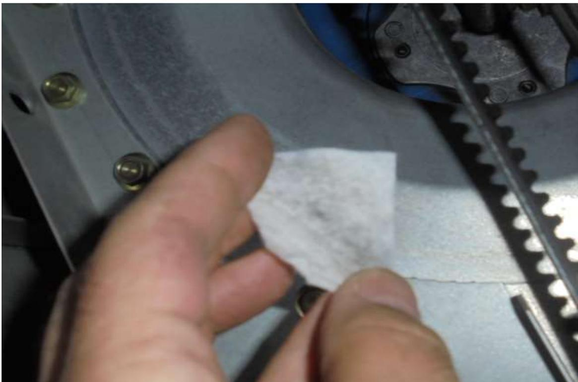
**Light Particulate Deposit Noted at Fan Inlet**
